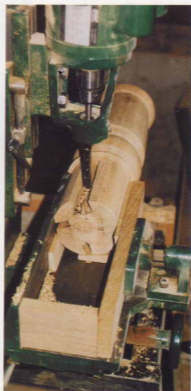
Chopping the leg sockets —Three tapered shims hold the column in register as a hollow-chisel mortiser cuts the cheeks of the dovetail sockets.
