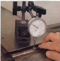
Setting jointer knives, p. 86
